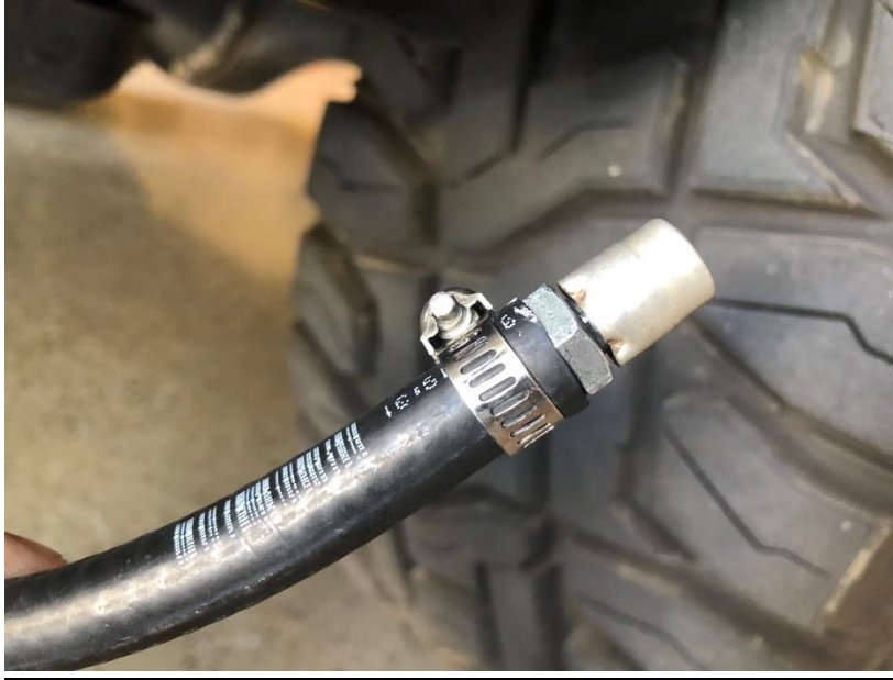
Figure 3 – Differential Breather Relocated to Provided Hose
