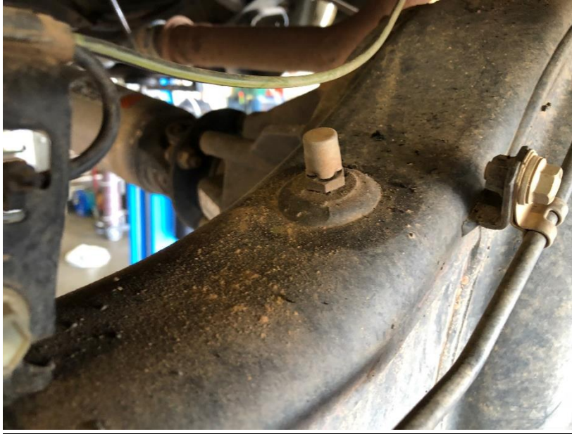
Figure 1 – Factory Differential Breather on Rear Differential
