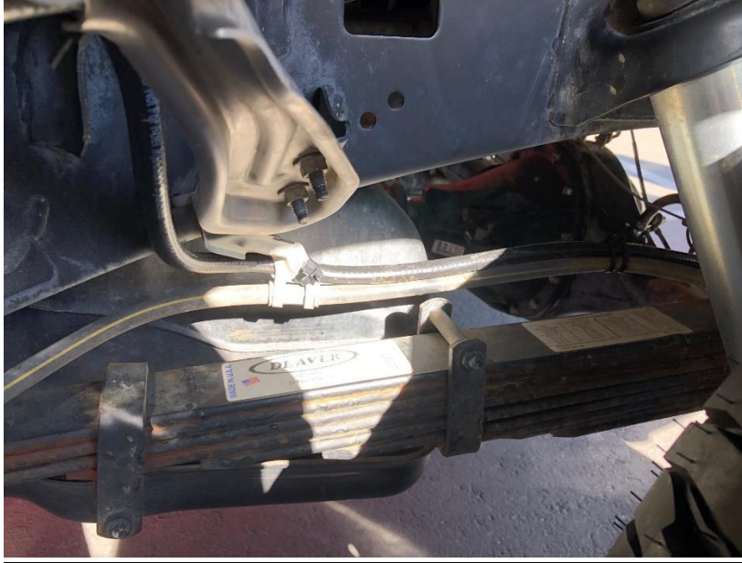
Figure 5 – Routing of Hose along Emergency Brake Line to Fuel Filler – Use Zip Ties
