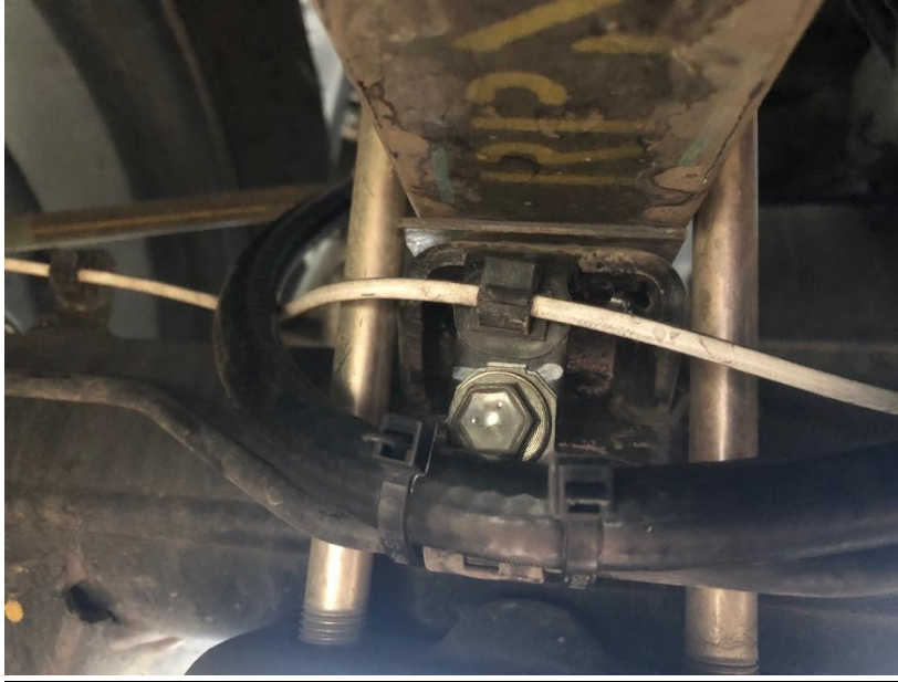
Figure 4 – Routing of Hose along Emergency Brake Line – Use Zip Ties
