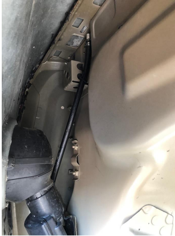
Figure 6 – Routing of Hose Behind Fuel Filler (Example) – Use Zip Ties Example Installation – Subject to Variances per Routing
