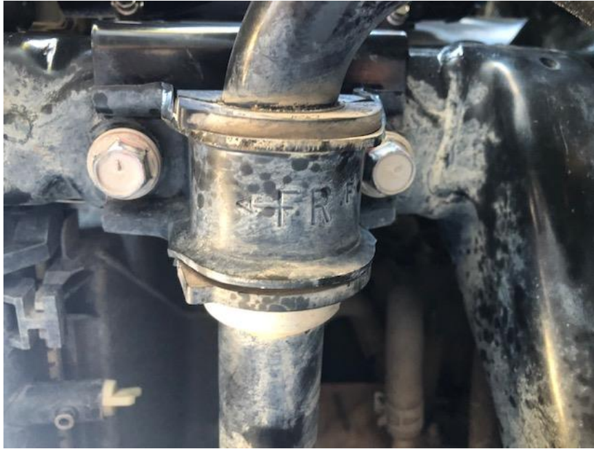
Figure 3 – Sway Bar Mounting Points (Loosen Only)
