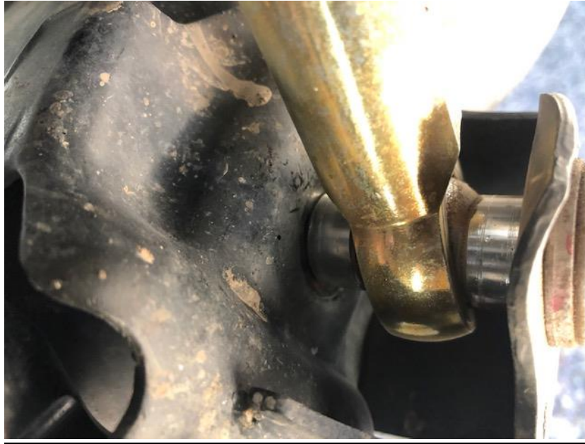
Figure 6 – Aligned and connected Upper Control Arm with Small Sleeves
